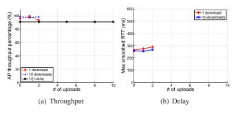
Fig. 18. Performance of the  $A^*$  algorithm for 802.11 DCF operation when there are both upload and download flows in the network. Here the AP throughput percentage is the ratio between the throughput achieved using the  $A^*$  algorithm and the maximum throughput using fixed size buffers. Physical layer data and basic rates used are 54 and 6 Mbps.
